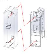
10. Check that the canopy seals are inserted correctly
