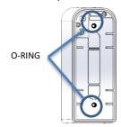
8. Drill the concentric seal and pass through the tamper cable
