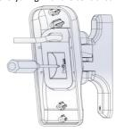
5. Remove the metal plate from the back of the transmitter holder
