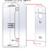
Check that the seals in the canopy are inserted correctly
